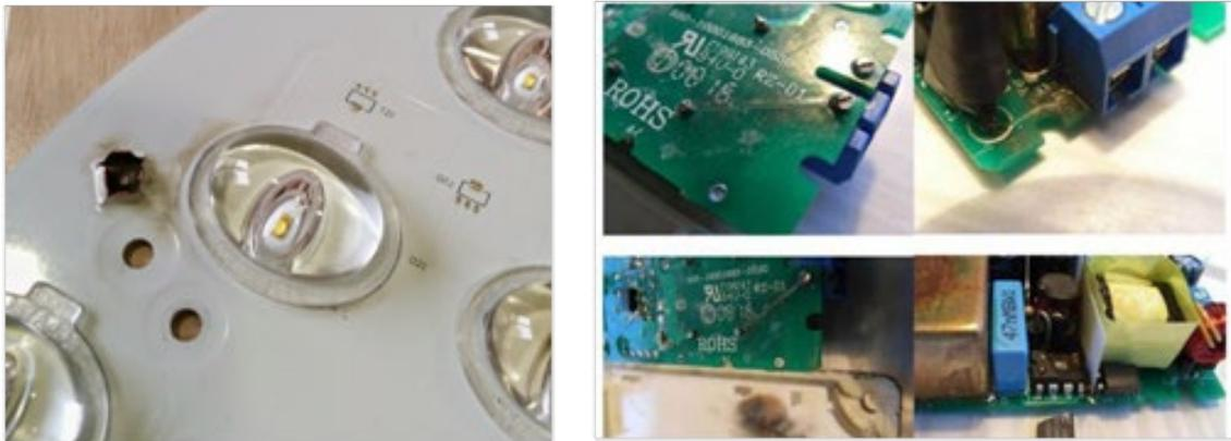
*Examples of destruction to LED arrays and drivers due to lightning surges*
